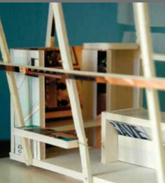
This is a model for a garden structure, made using recycled mounting board and dress making pins - it is rudimentary yet not crude. It serves an important purpose when explaining the steel framing to the contractor.
