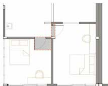
Diagram showing how the threshold to a room changes with the door swing.
