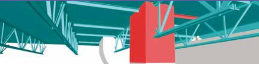
Figure 1 Detecting structural clashes in your model in design development stage before it goes to construction. Source: McGraw-Hill.
